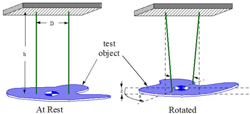
**Figure 2.7.3-2 Bifilar Torsional Pendulum (mathworks.com)**
